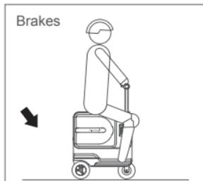
Turn the brake lever to brake
