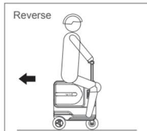
Turn the brake switch and turn it off and then turn the acceleration switch to reverse
